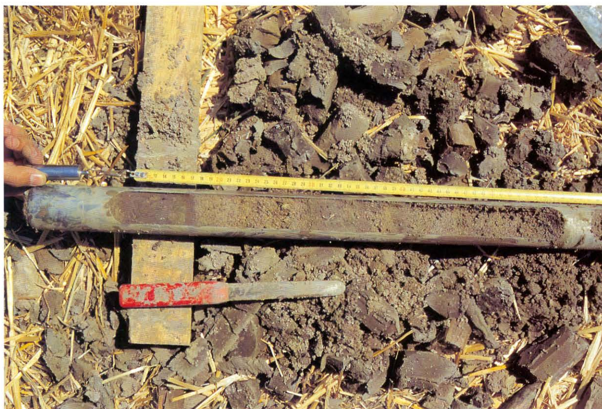
Fig. 10 A gouge-auger sample from drillhole number 117 at a depth of 950–1000 cm. Darker-finer-cohesive and lighter-coarser-looser sediment bands indicate a fluctuating, unstable environment. This section coincides with the end of the marine sequence, and belongs to a deltaic-coastal environment.
