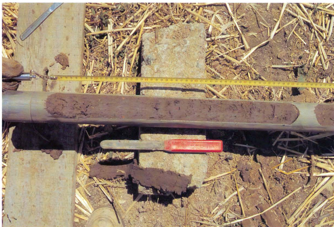
Fig. 11 A gouge-auger sample from drillhole number 101. It is taken from 300–350 cm below present surface by percussion drilling. A sample is taken from a colluvial sediment unit which contains a high density of small grains of sherds, charcoal, and marine shells (remains of food). This unit covers a fairly wide area to the south of the Lower City.
